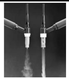
A collet body with a gas lens can be very useful to a welder. The purpose of a gas lens is to make the shielding gas exit the nozzle as a column instead of as a turbulent stream of gas that begins to spread out after exiting. The column of gas allows the electrode to stick out farther for visibility, allowing for better access to the weld area, and a reduction in gas flow (CFH/L/Min).
